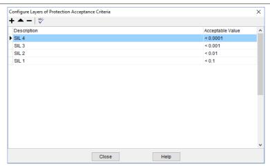
Whatever the acceptance criteria used BowTie Pro™ will display if the criteria is Met by displaying a red or green bar at the bottom of the screen and the Consequence box on the diagram.
