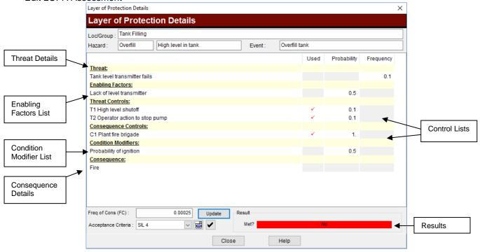
The screen allow the entry of the information as detailed in the LOPA overview with the results being displayed at the bottom.
