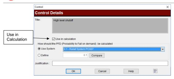
The control can have a Probability of Failure on Demand (PFD). The PFD is independent of the other controls on similar branches eg the same control but leading to a fire rather than a Spill may have a different value
