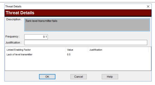
The description is read-only and the Frequency is now a mandatory value. This is the same as the value entered on the bowtie Threat screen and is defined as the Frequency of the Threat occurring per year, in this example  $10^{-1}$  (0.1). Ideally a justification for this Frequency should also be provided.
