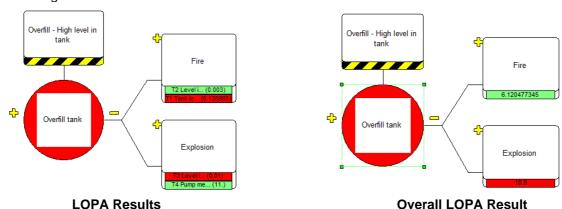
The LOPA Results show the result of the branch-by-branch analysis as described above. The Overall LOPA result is determined on a screen which is accessed by right clicking on the Consequence and selecting "Overall LOPA Consequence".
