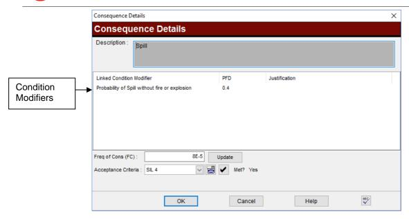
From this screen it is possible to add many Condition Modifiers. A condition modifier is used to determine the probability of a specific event, eg in this example if there is a release of oil what is the probability of it just spilling rather than causing a fire. The list of used Condition Modifiers is displayed in the middle of the screen and additional Condition Modifiers can be added to the branch by selecting the grid and pressing "New" from the popup menu.
