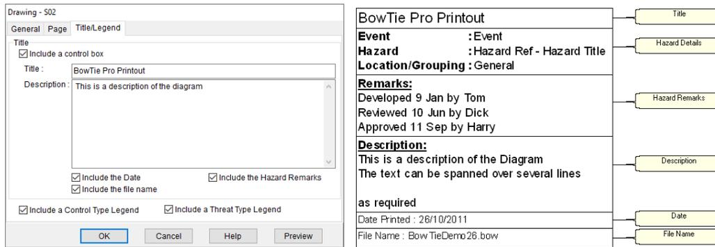
Ability to add a threat types and control types legend to the bottom of the diagram. This gives definition to the colours used on the output.
